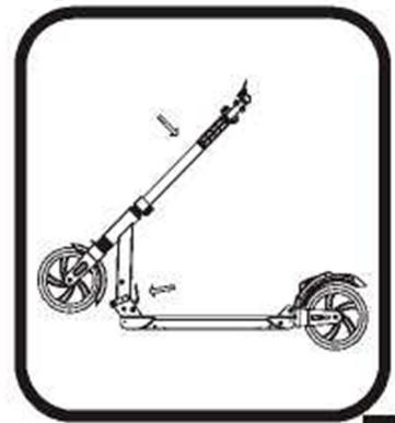
Push the folding button upwards and pull the handle bar downwards. When you sounds clicks, the scooter is completely folded.
